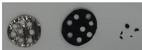
Figure 43: Samples of substrates. Left: uncoated, corrugated disk; Center: coated, corrugated disk; Right: coated punch-out.
