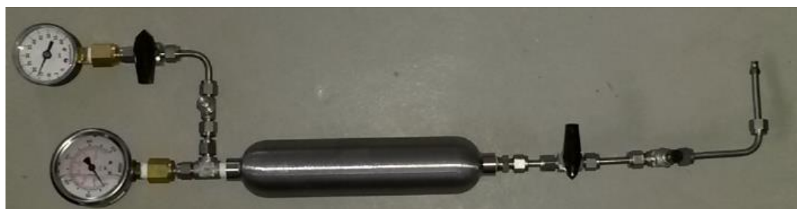
Figure 44: Calibration bomb used for microGC calibration equipped with a high pressure gauge and isolated low pressure gauge.
