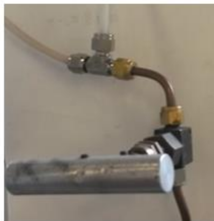
Figure 42: metering valve towards furnace purge.
