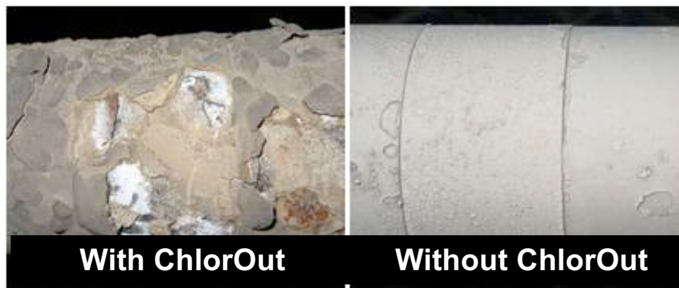
Figure 3-4. Boiler tubes without and with Chlorout injection [80].
