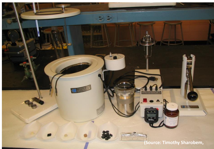
Figure 12: Experimental setup - Parr oxygen bomb calorimeter
